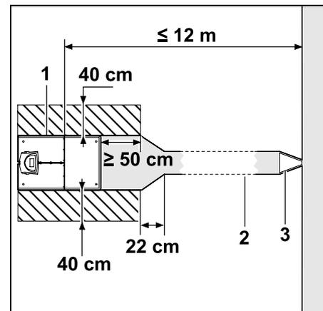
The docking station (1) can be installed as illustrated with a corridor (2) for docking and undocking to take place correctly. The areas around the docking station and outside of the perimeter wire must be flat and freely travelable. Remove any bumps or depressions.
