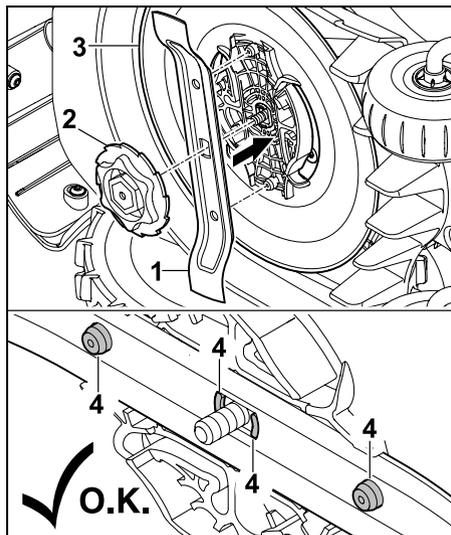
Fit the mowing blade (1) and fastening nut (2) on the carrier plate (3) as illustrated. Ensure the correct position of the retainers (4) in the mowing blade.
