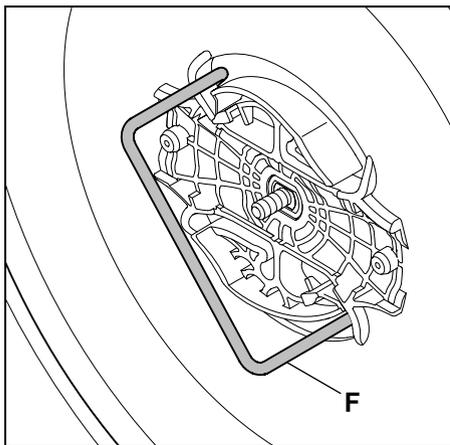
Insert the puller (F) and turn anti-clockwise to the stop.
