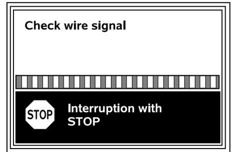
Checking the wire signal may take several minutes. The red STOP button on top of the machine terminates the link, the previous installation assistant step is called up.
