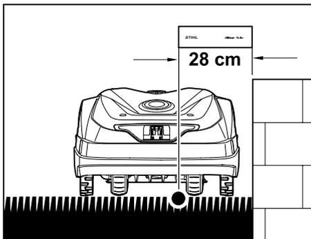
The robotic mower must run completely within the mowing area and must not touch the obstacle.
