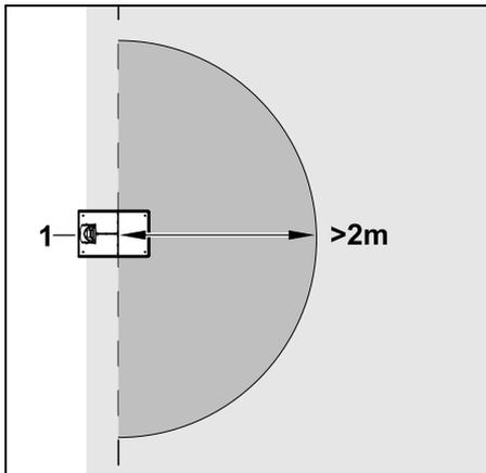
In order for docking to take place smoothly, no no-go area must be installed within a radius of at least **2 m** around the docking station (1).
