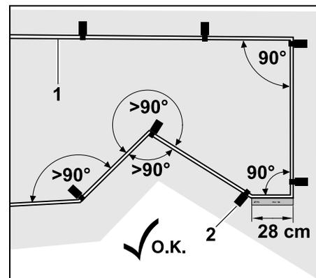
Avoid routing at acute angles (less than 90°). In acutely angled lawn corners, fasten the perimeter wire (1) to the ground with fixing pins (2) as illustrated. (⇒ 12.6)
