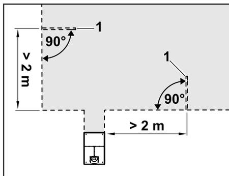
Guide loops must not be installed in the vicinity of corners.
