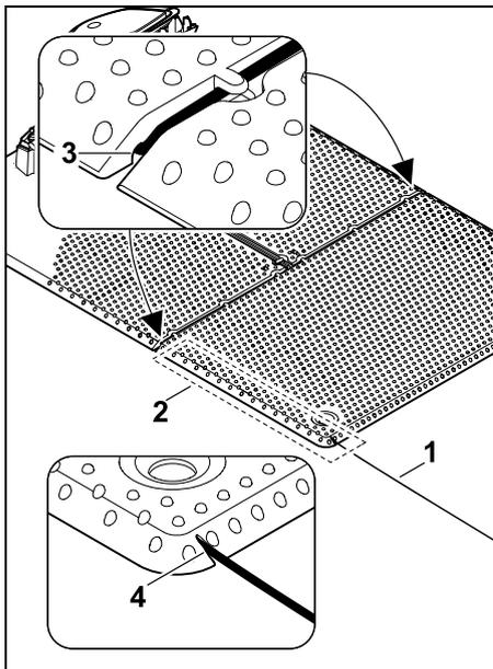
Route the perimeter wire (1) in the area (2) under the floor plate. To do this, guide the wire into the wire outlets (3, 4) – loosen the pegs if necessary.
