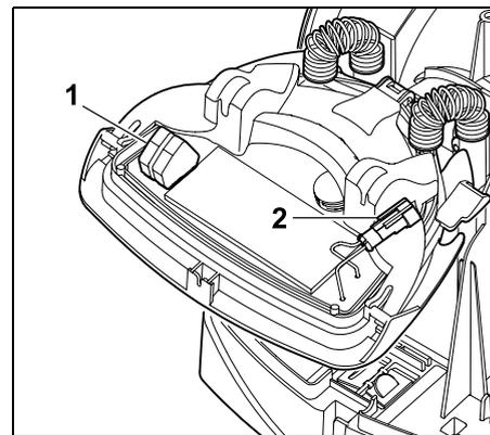
The connections for the perimeter wire (1) and the power cable (2) are protected against the weather when the panel is closed.
