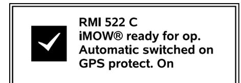
The name of the robotic mower (⇒ 10.) and the text "iMOW® ready for op." are displayed in the bottom area of the screen together with the symbol shown, the automatic mowing status (⇒ 15.4) and information on GPS protection (⇒ 5.9).
