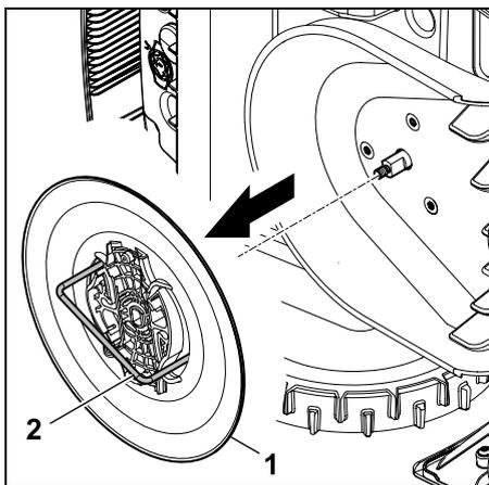
Support the machine with one hand. Remove the carrier plate (1) by pulling on the puller (2).
