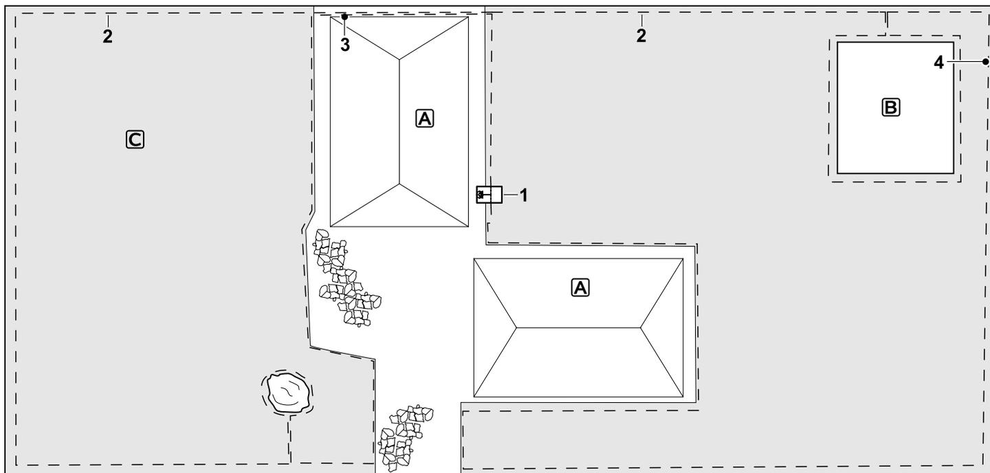
Divided mowing area – the robotic mower cannot travel independently from one mowing area to the other.
