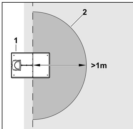
There must be a free, level area (2) with a radius of at least 1 m in front of the docking station (1). Remove any bumps or depressions.
