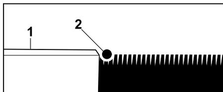
Height difference to obstacle that can be travelled on (1) is less than +/- 1 cm: route the perimeter wire (2) without clearance to the obstacle.
