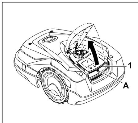
Grasp the flap (1) at the lifting point (A) and release upwards by pulling lightly. Open the flap as far as the stop.
