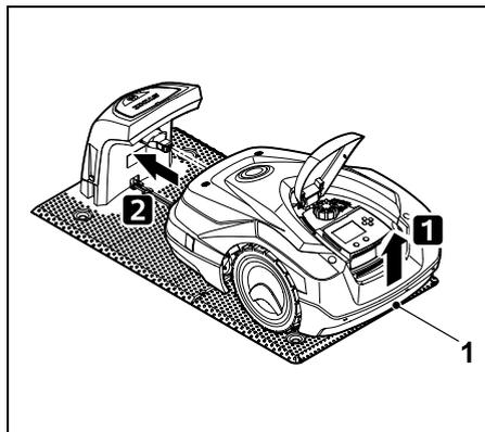
Lift the robotic mower slightly by the carrying handle (1) to relieve the weight on the drive wheels. Push the machine, resting on its front wheels, into the docking station.
