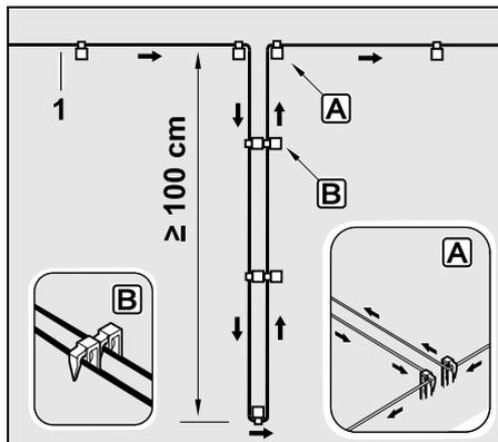
Install the guide loop in the mowing area as shown. The perimeter wire (1) must be fastened to the ground with two fixing pins at the edge **A** and must not be crossed.
