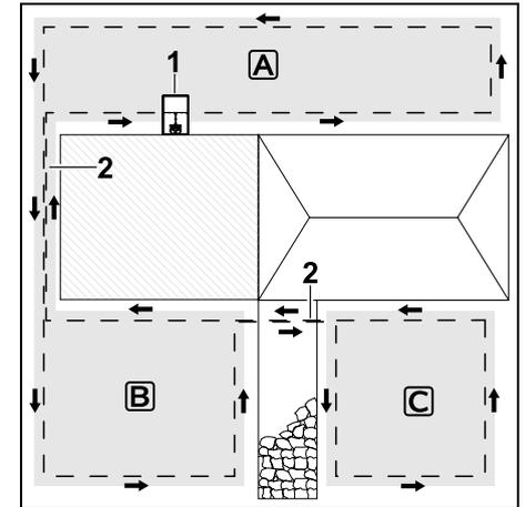
The docking station (1) is installed in the mowing area **A**, which is cut fully automatically in accordance with the mowing plan.
