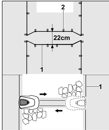
In corridors, the perimeter wire (1) must be routed parallel and attached to the ground with a sufficient number of fixing pins (2). At the start and end of the corridor, funnel-shaped entrance and exit areas must be installed.
