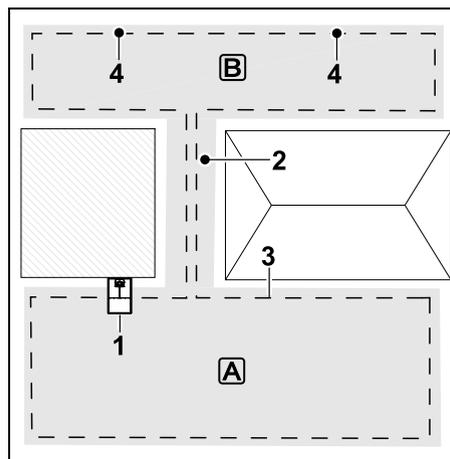
The docking station (1) is installed in mowing area **A**. Mowing area **B** is linked to mowing area **A** by means of a corridor (2). The perimeter wire (3) can be continuously followed by the robotic mower. In order to mow mowing area **B**, starting points (4) must be defined. (⇒ 11.14)
