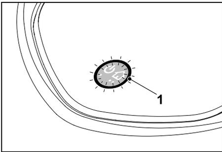
When the perimeter wire is correctly installed and the docking station is connected to the mains power supply, the LED (1) illuminates.
