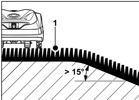
If there is a slope with an incline > 15° on which a perimeter wire is to be installed in the mowing area, it is recommended that the perimeter wire (1) be routed in the flat area before the top edge of the slope. The top edge and area of the slope are not mown.
