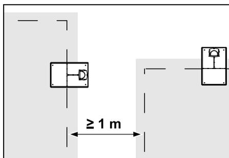
Mowing areas must not overlap. Maintain a minimum clearance of  $\geq 1$  m between the perimeter wires of two mowing areas.
