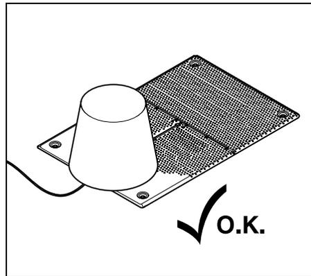
Cover the docking station with a suitable bucket, fasten the bucket in place.
