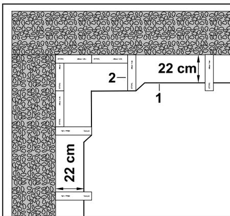
Route the perimeter wire (1) as illustrated at the internal corner. Use the iMOW® Ruler (2).
