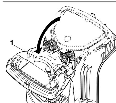
Fold the panel (1) forwards. Hold the panel in the opened position as the hinge springs will close it automatically.
