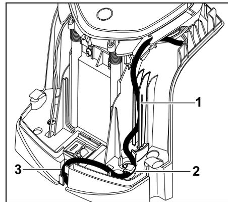
Press the power cable into the cable guide (1) as illustrated and guide through the strain relief (2) and the cable duct (3) to the power supply unit.
