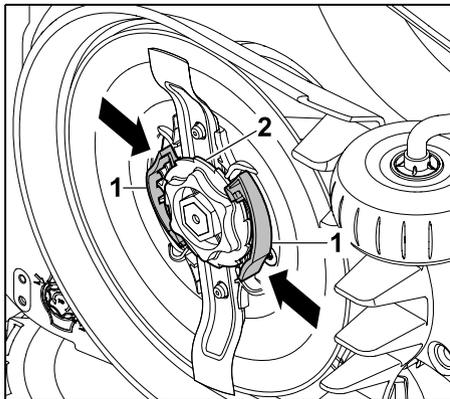
Push in both tabs (1) on the carrier plate with one hand and hold. Remove the fastening nut (2) with your other hand. Remove the mowing blade together with the fastening nut.
