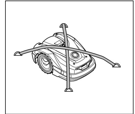
Secure the robotic mower on the load floor. Fasten the machine as illustrated using suitable fastening materials (straps, ropes) for this purpose.
