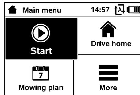
The main menu comprises 4 submenus, displayed as buttons. The selected submenu has a black background and is opened using the OK button.
