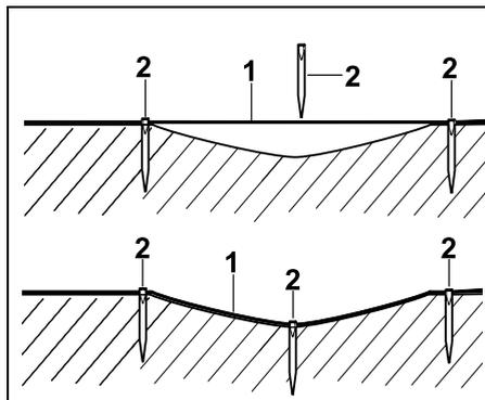
The perimeter wire (1) is routed above ground and attached with additional fixing pins (2) in case of unevenness. This prevents the wire being cut by the mowing blade.
