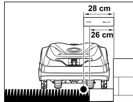
Route the perimeter wire at a clearance of 28 cm to the obstacle. To ensure that the lawn edge is mown completely, the edging stones must have a width of at least 26 cm. If wider edging stones are laid, the lawn edge is cut even more precisely.
