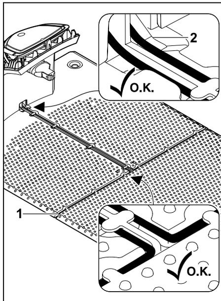
Insert the perimeter wire (1) into the cable guides in the floor plate and guide it through the socket (2).
