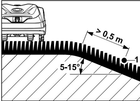
If there is a slope with an incline of 5° - 15° in the mowing area, the perimeter wire can be routed below the top edge of the slope in the slope as illustrated. The minimum clearance (0,5 m) from the top edge of the slope to the perimeter wire must be taken into account for trouble-free operation of the robotic mower.
