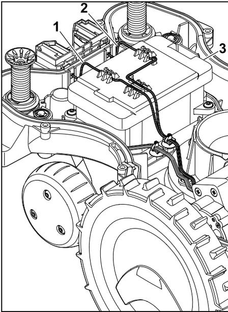
Remove cable (1) and cable (2) from the cable guides and remove the battery (3).
