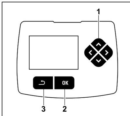
The control pad comprises four direction buttons (1). It serves for navigation in the menus. Settings are confirmed and menus opened using the OK button (2). Menus can be exited again using the Back button (3).
