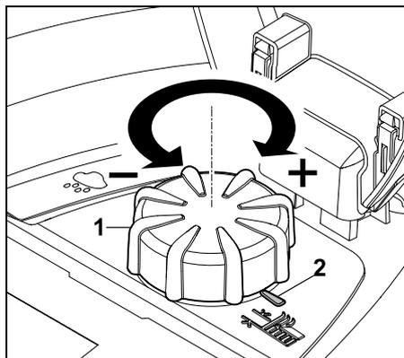
Turn the rotary knob (1). The marking (2) indicates the set cutting height.
