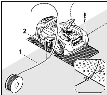
Fasten the perimeter wire (1) to the ground on the **left or right** as appropriate, next to the floor plate, directly next to a wire outlet, using a fixing pin (2).
