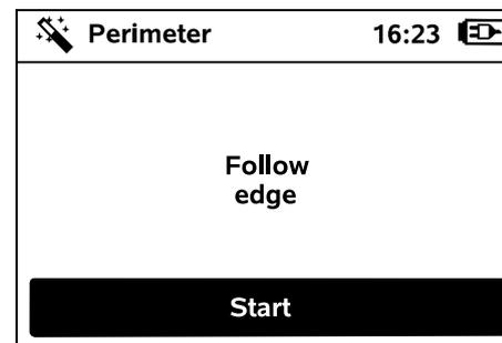
Start edge following by pressing the OK button – this does not activate the mowing blade.
