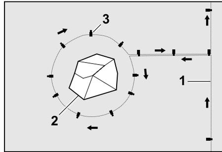
Route the perimeter wire (1) from the edge to the obstacle with the correct clearance around the obstacle (2) and attach it to the ground with a sufficient number of fixing pins (3). Then route the perimeter wire back to the edge again.
