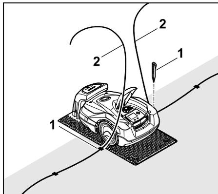
Drive in the last fixing pin (1) on the left or right next to the floor plate, directly next to the wire outlet. Cut off the perimeter wire (2) to a free length of approx. 1.5 m.
