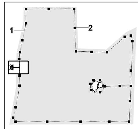
Route the perimeter wire (1) around the mowing area and around any obstacles (⇒ 12.9) and fasten it to the ground using fixing pins (2). Check the clearances using the iMOW® Ruler. (⇒ 12.5)
