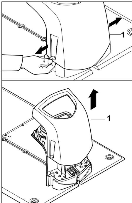
Pull the cover (1) apart slightly on the left and right as illustrated and remove upwards.
