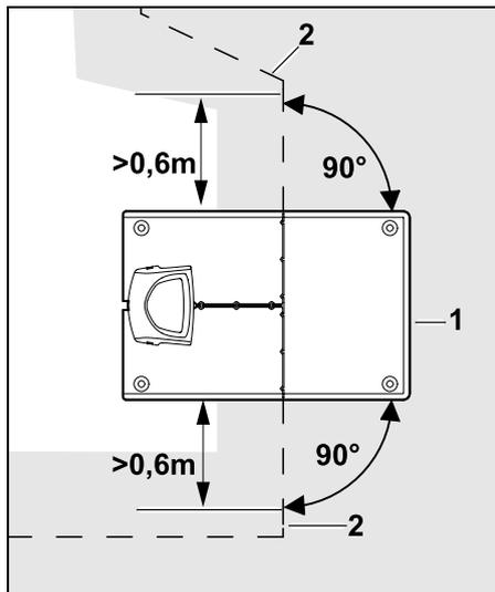
Route the perimeter wire (2) in front of and behind the docking station (1) for **0.6 m** in a straight line and at right angles to the floor plate. Then follow the edge of the mowing area with the perimeter wire.
