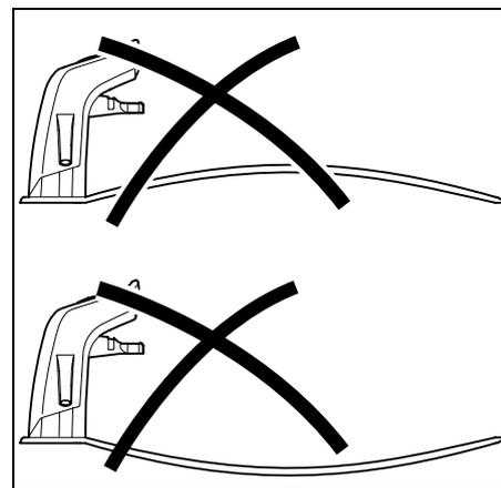
Never bend the floor plate. Any unevenness must be removed under the floor plate so that it fully contacts the ground.
