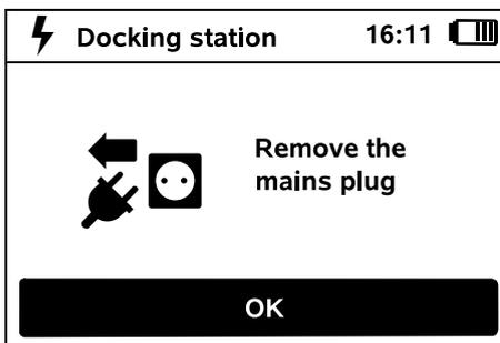
Disconnect the power supply unit plug from the mains, then press the OK button.
