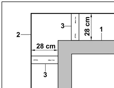
When routing around high obstacles such as wall corners or high flowerbeds (1), the wire clearance must be maintained at the corners to prevent the robotic mower from scraping against the obstacle. Route the perimeter wire (2) with the aid of the iMOW® Ruler (3) as illustrated.
