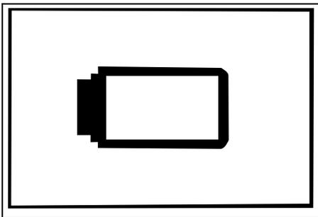
If the battery charge is too low, the corresponding battery symbol appears. In this case, place the robotic mower in the docking station to recharge.
