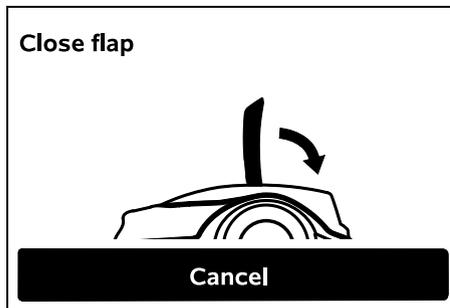
Close the flap of the robotic mower. (⇒ 15.2) Only once the flap has been closed does the robotic mower start automatically and follow the edge along the perimeter wire.
