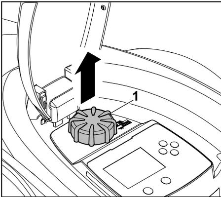
Remove the rotary knob (1) upwards.
