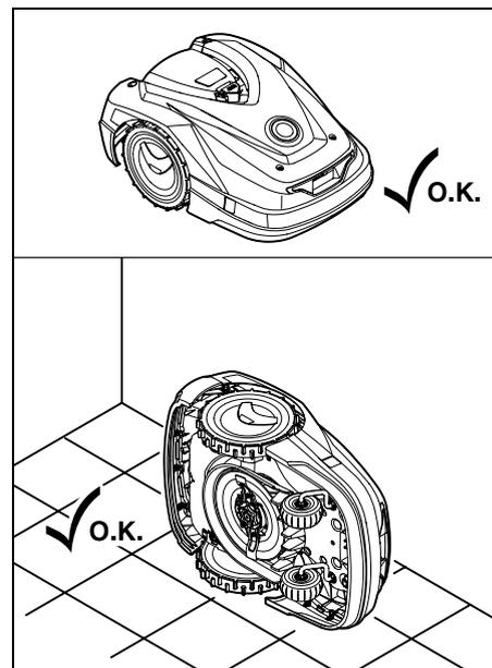
Place the machine on a firm, level and flat surface for cleaning the **top of the machine** (hood, flap). To clean the
