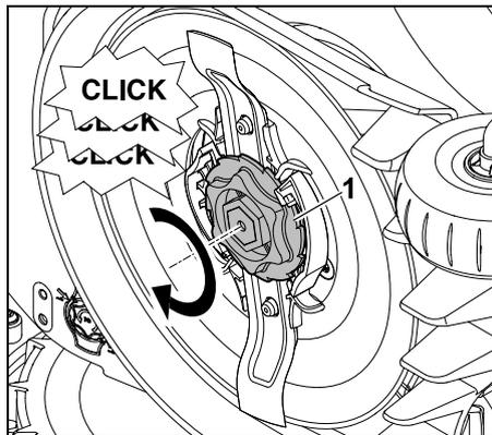
Screw on the fastening nut (1) as far as possible. Several clicks are audible during tightening. Ensure secure seating of the mowing blade by shaking carefully.
