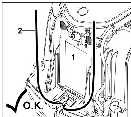
Shorten the left wire end (1) and right wire end (2) to the same length. Length from the wire outlet to the wire end: **40 cm**
