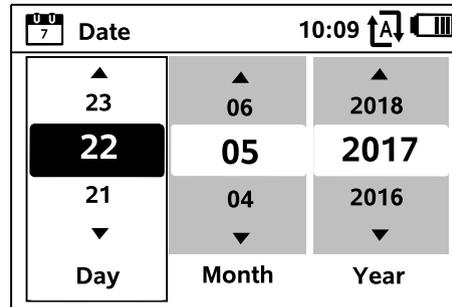
Settings can be changed by pressing the control pad. The current value is highlighted in black. The OK button confirms all the values.
