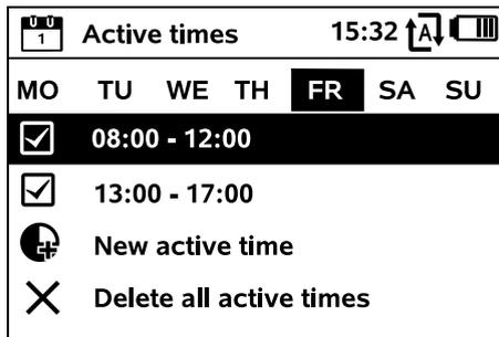
Mowing is permitted during **ticked** active times; these times are marked in black in the mowing plan.
