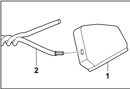
Thread a grommet (1) onto each of the two wire ends (2).
