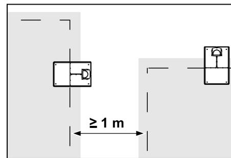
Mowing areas must not overlap. Maintain a minimum clearance of **≥ 1 m** between the perimeter wires of two mowing areas.
