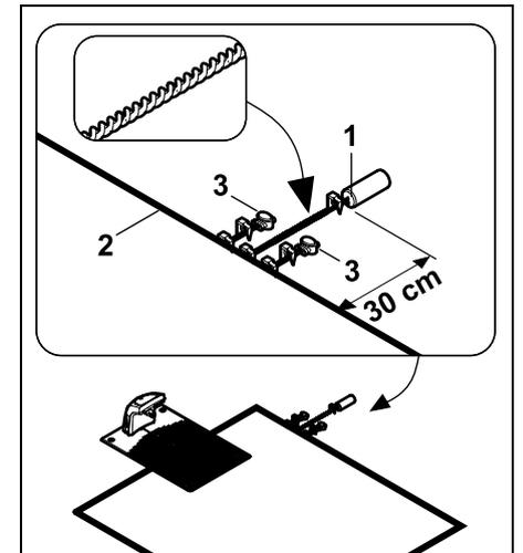
Fasten the AKM 100 (1) 30 cm outside the mowing area using a fixing pin. Twist the wire ends as far as the mowing area and fasten using a fixing pin.
