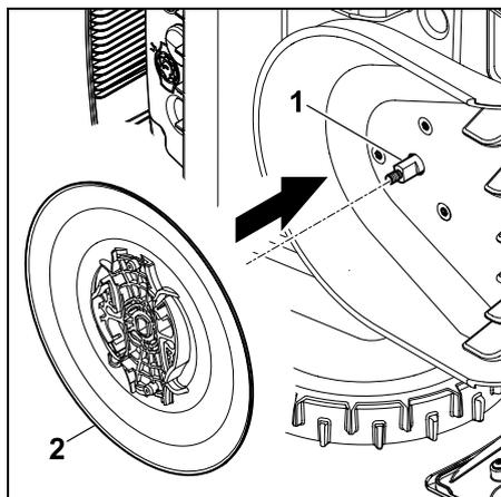
Thoroughly clean the blade shaft (1) and the mounting on the carrier plate (2). Push the carrier plate as far as possible onto the blade shaft.
