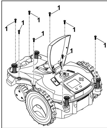
Unscrew the screws (1) and remove.
