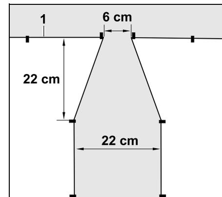
The perimeter wire (1) must be routed in a funnel shape as illustrated at the start and end of a corridor. This prevents the robotic mower from accidentally driving into the corridor during mowing.
