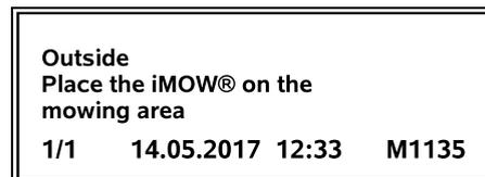
Errors, faults or recommendations are displayed together with warning symbol, date, time and message code. If several messages are active, they appear alternately. (⇒ 24.)
