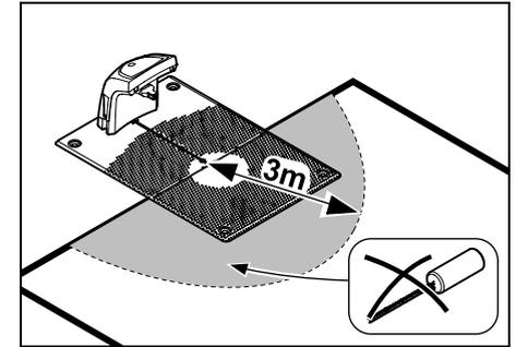
Install the AKM 100 with a minimum clearance to the docking station of 3 m.
