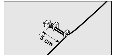
Attach the perimeter wire strain relief to the ground with two fixing pins as illustrated.
