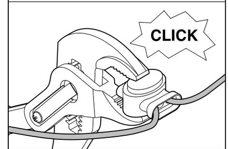
Insert loose, unstripped wire ends (1) to the stop in the wire connector (2). Press the wire connector together using suitable pliers – ensure correct engagement.
