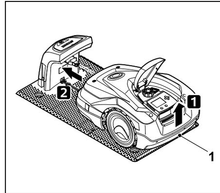
Lift the robotic mower slightly by the carrying handle (1) to relieve the weight on the drive wheels. Push the machine, resting on its front wheels, into the docking station.
