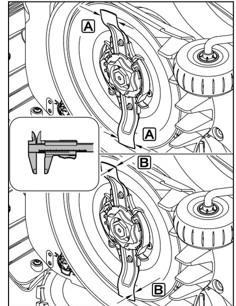
Check the **blade width** **A** and **blade thickness** **B** using a slide caliper. If the blade width is less than **25 mm** or the blade thickness is less than **1,3 mm** at any point, the mowing blade must be replaced.
