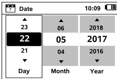
Set the current date using the control pad and confirm with the OK button. **OK**
