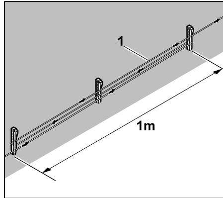
Route perimeter wire (1) as illustrated between 2 fixing pins spaced approx. 1 m apart. Attach the reserve wire to the ground in the centre using a further fixing pin.
