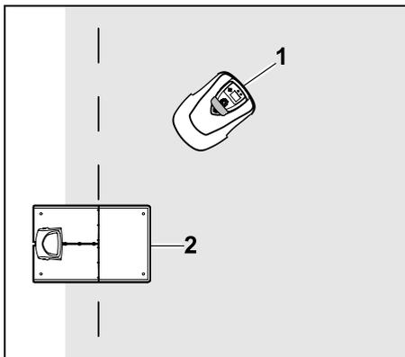
Place the robotic mower (1) within the mowing area, behind the docking station (2) as illustrated, then press the OK button.
