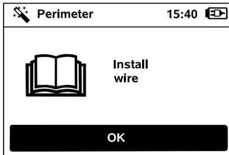
Route the perimeter wire starting at the docking station. A distinction must be made between an **internal docking station** and an **external docking station** here.
