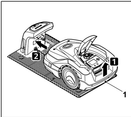
ic mower slightly by the carrying handle (1) to relieve the weight on the drive wheels. Push the machine, resting on its front wheels, into the docking station.
