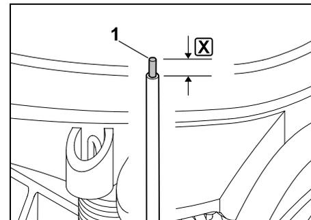
Strip the left wire end (1) to the specified length **X** using a suitable tool and twist the wire strands.
