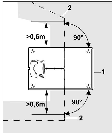
Route the perimeter wire (2) in front of and behind the docking station (1) for **0.6 m** in a straight line and at right angles to the floor plate. Then follow the edge of the mowing area with the perimeter wire.
