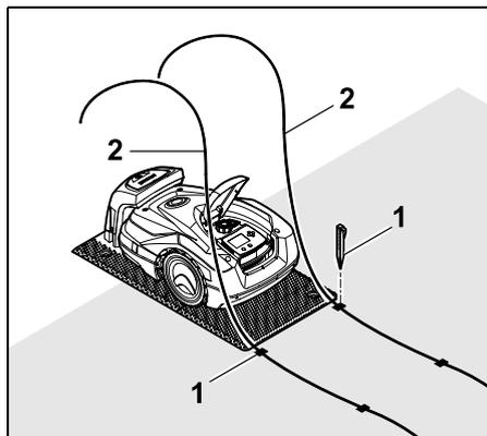
Drive in the last fixing pin (1) on the left or right behind the floor plate, directly next to the wire outlet. Cut off the perimeter wire (2) to a free length of approx. 2 m.
