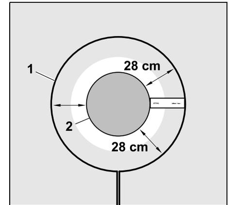
The robotic mower travels along the perimeter wire (1) around the obstacle (2) without bumping into it.
