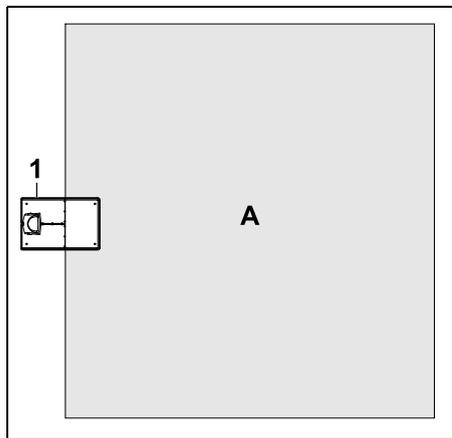
The docking station (1) is installed within the mowing area (A), right at the edge.
