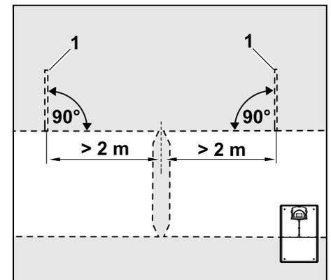
To the right and left of the corridor access, two guide loops (1) have to be installed at an angle of 90° to the perimeter wire.
