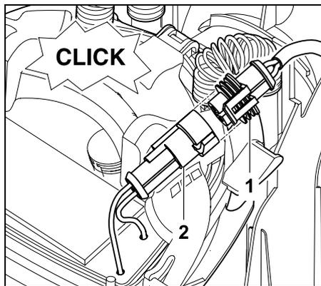
Connect the connector of the power supply unit (1) to the connector of the docking station (2).
