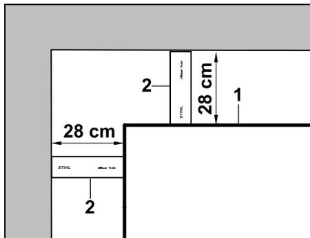
When routing the perimeter wire (1) at an internal corner at a high obstacle, measure the wire clearance with the iMOW® Ruler (2).
