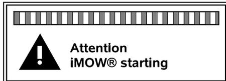
The text "Attention – iMOW® starting" and a warning symbol are displayed **before the mowing operation**.
