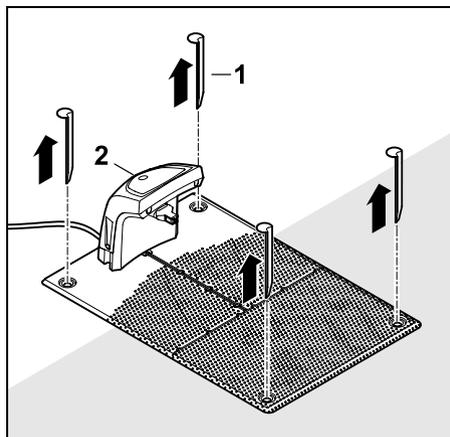
Pull out the pegs (1), remove the docking station (2) from the lawn with the power supply unit connected, clean thoroughly (with a moist cloth) and put into storage.
