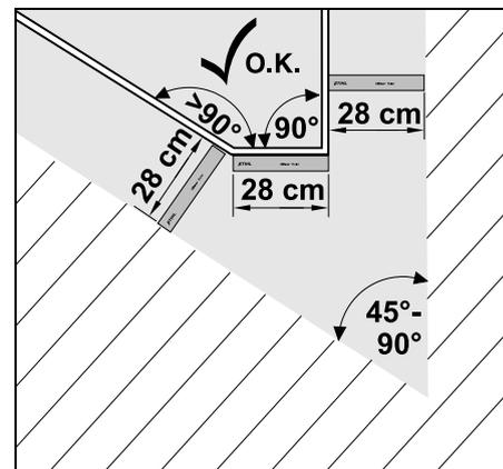
The perimeter wire is routed as illustrated in acutely angled lawn corners (45° - 90°). The two angles must have a clearance of at least 28 cm so that the robotic mower can follow the edge.
