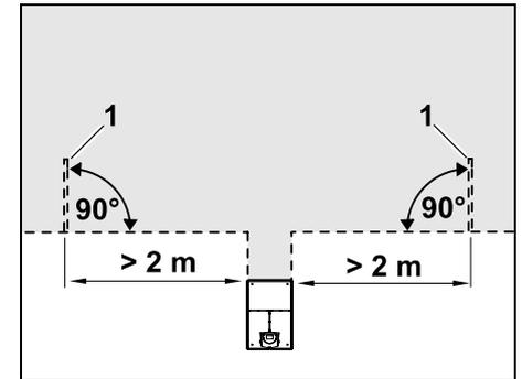
To the right and left of the access to the external docking station, two guide loops (1) have to be installed at an angle of 90° to the perimeter wire. Minimum clearance to access: **2 m**
