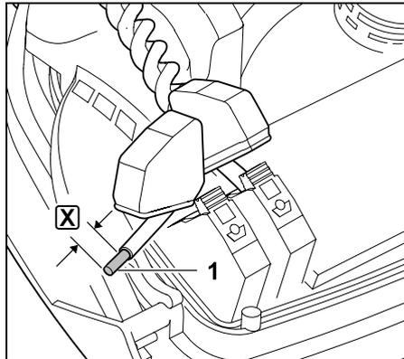
Strip the right wire end (1) to the specified length **X** using a suitable tool and twist the wire strands.
