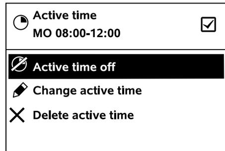
The selected active time for automatic mowing can be disabled or enabled using **Active time off**
