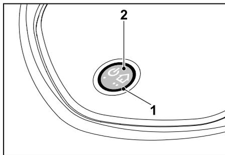
A circular red LED (1) provides information on the status of the docking station and the wire signal.
