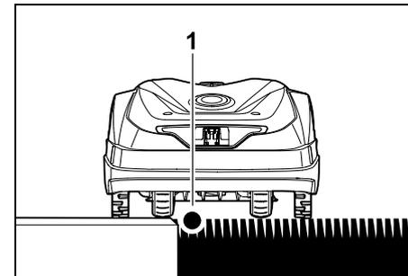
The perimeter wire (1) can be routed **without clearance** along obstacles that can be travelled on such as patios and paths. The robotic mower then travels with one rear wheel outside the mowing area. Maximum stepped area to the turf: **+/- 1 cm**
