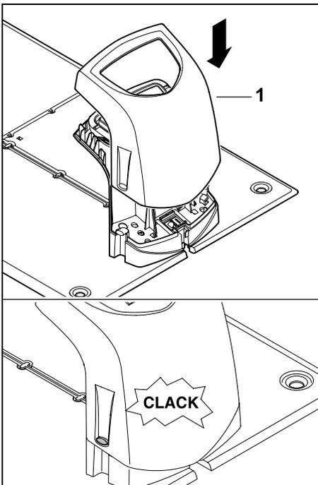
Fit the cover (1) onto the docking station and allow it to engage – do not pinch any cables.
