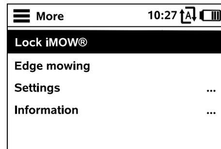
The second menu level is displayed as a list. You move up and down through the submenu by pressing the control pad. Active menu entries have a black background.
