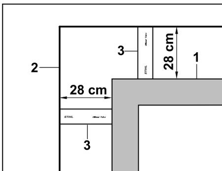
When routing around high obstacles (1) such as wall corners or high flowerbeds, the wire clearance must be maintained at the corners to prevent the robotic mower from scraping against the obstacle. Route the perimeter wire (2) with the aid of the iMOW® Ruler (3) as illustrated.
