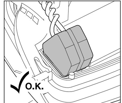
Fit the grommets over the terminal blocks.
