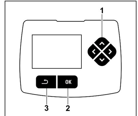
The control pad (1) serves for navigation in the menus. Settings are confirmed and menus opened using the OK button (2). Menu can be exited again using the Back button (3).
