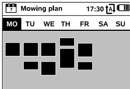
The **saved mowing plan** can be called up via the "Active times" menu in the "Mowing plan" menu. The rectangular blocks beneath the respective days represent the saved active times. Mowing is possible in active times marked in black. Grey blocks represent active times without mowing operations – e.g. in the case of a disabled active time.
