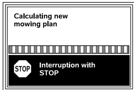
A new mowing plan is being calculated. The procedure can be cancelled using the red STOP button on the top of the machine.
