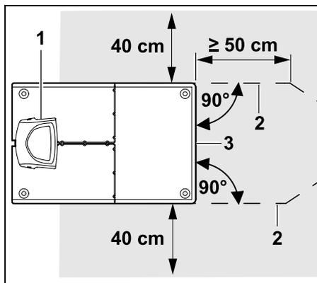
Route the perimeter wire (2) in front of and behind the docking station (1) with 50 cm of clearance and at right angles to the floor plate. A corridor can then be installed (⇒ 12.11) or the edge of the mowing area followed with the perimeter wire.
