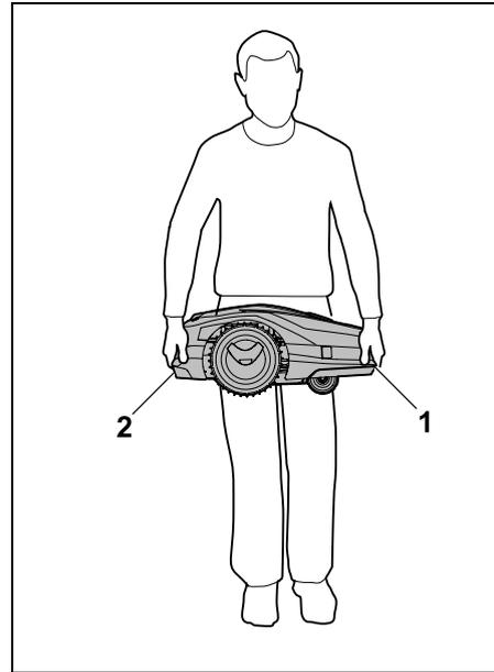
Lift and carry the robotic mower at the front carrying handle (1) and at the rear carrying handle (2). Ensure that the mowing blade always faces away from your body and that there is sufficient distance between the mowing blade and body, particularly the feet and legs.
