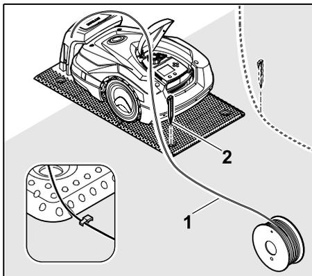
Fasten the perimeter wire (1) to the ground on the **left** or **right** as appropriate, behind the floor plate, directly next to a wire outlet, using a fixing pin (2).
