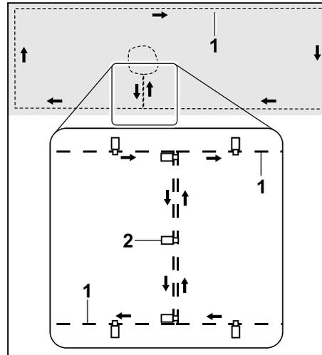
In linking sections, the perimeter wire (1) must be routed parallel, the wires must not cross and must be close to one another. Attach the linking section to the ground with a sufficient number of fixing pins (2).
